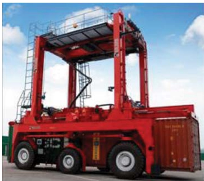
Automated Shuttle Carrier (AShC) Fuente: AShC de la casa KALMAR operando el puerto de Fisherman Island Terminal, Brisbane, Australia. http://www.cidesport.com.br
